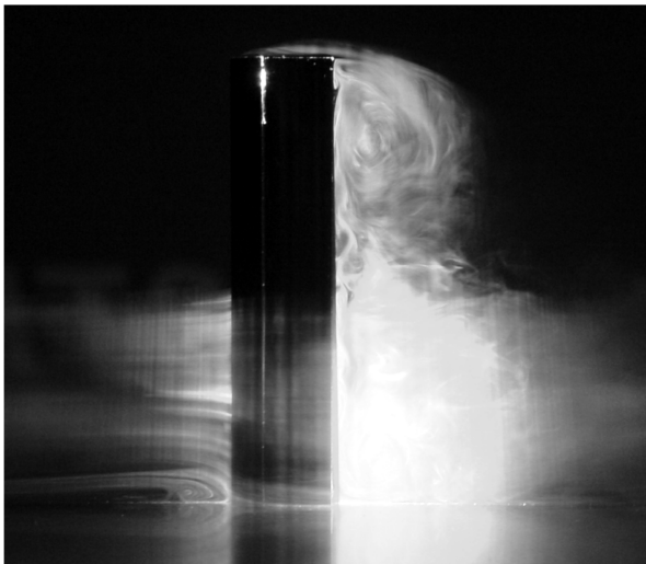
Fig. 20 Flow visualization, velocity distribution, and turbulent kinetic energy for a) unmodified cylinder, b) cylinder with an elliptical afterbody, and c) cylinder with a wedge in front ( U_0 = 10 m/s).
